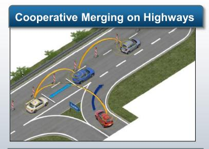
Based on notification of intended merging, interested vehicles exchange info to coordinate gap opening and merging maneuvers with increased time spans
