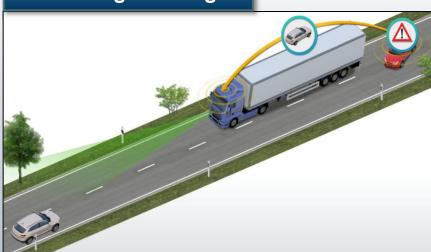
Overtaking car analyses the rx info and warn the driver if necessary
