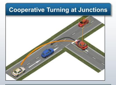
Based on notifications of intended turning, interested vehicles exchange info to coordinate right of way and transit maneuvers with increased time spans
